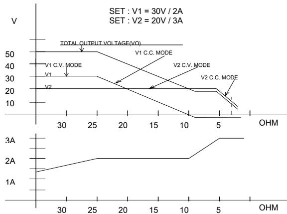
Figure 5 Serial Voltage/Current Output vs. Load Change
