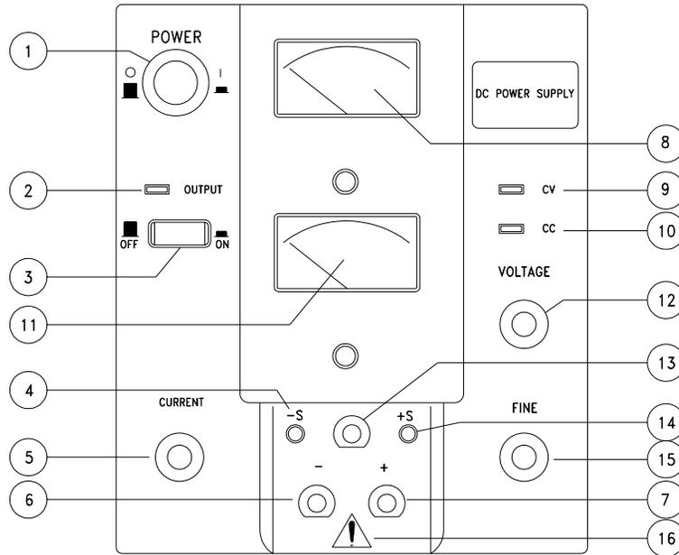
Front panel with analog meter for models 3203AR, 3302AR, 3303AR and 3601AR
