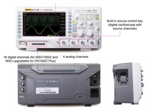
Product Dimensions: Width×Height×Depth=313.1 mm×160.8 mm×122.4 mm Weight: 3.2 kg  $\pm$  0.2 kg(Without Package)
