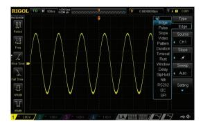
Built-in dual-channel 25 MHz source (DS1XX4Z-S Plus)
