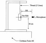
1 METER FROM MICROPHONE TO FAN INTAKE THE FAN IS RUNNING IN FREE AIR UNDER SHAFT HORIZONTAL CONDITION WITH THE MICROPHONE AT DISTANCE OF ONE METER FROM THE FAN INTAKE.
