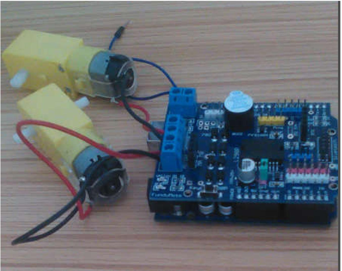
With wiring as the image shows, we can control forward rotation, reverse rotation, stop and the PWM speed of the two DC motors.
