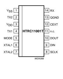
Fig.2 Pin configuration.
