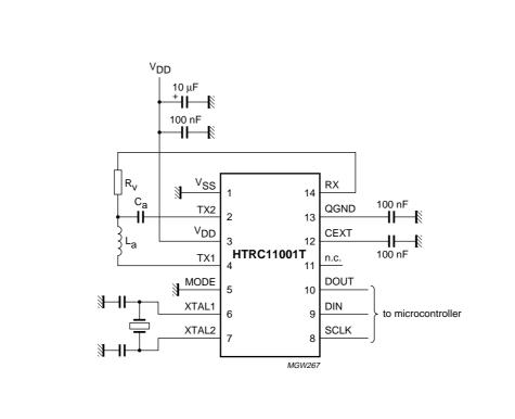
Fig.4 Minimum application circuitry.
