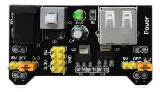
**KEYES MD0111** power module exclusive for breadboard/black breadboard power module (excluding breadboard)
