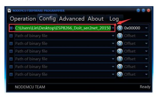
c. Click **Operation**, click on Flash(F), press the RST button, then press the KEY button, starting to burn the firmware as shown below.
