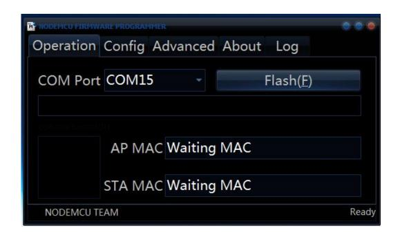
b. Click Config, select the firmware, and firmware version is ESP8266\_Doit\_ser2net\_20150723.
