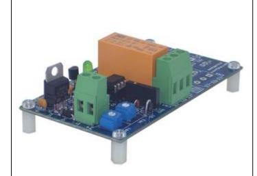
The **MEK06-001** is one in a sequence of controller based kits developed for a number of applications requiring some sort of input control, over one of the outputs that is either switched (ON-OFF) or PWM controlled, according to the input variable and a given function.
