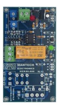
The controller requires 12VDC ( 10 to 14VDC ), which must be connected to the +V1 and GND terminals. Polarity must be observed.
