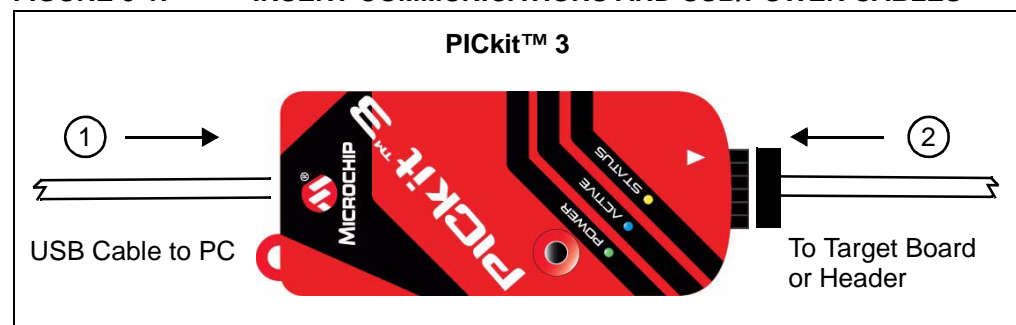
FIGURE 3-1: INSERT COMMUNICATIONS AND USB/POWER CABLES
