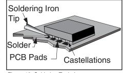
Figure 18: Soldering Technique
