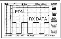
Figure 4: Turn-On Time from PDN
