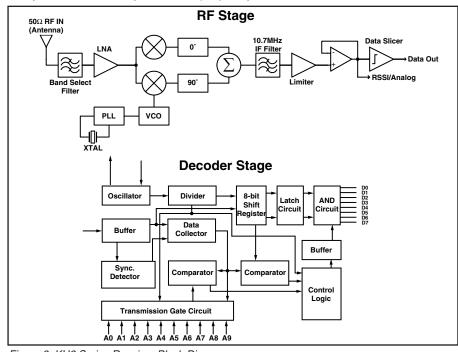
Figure 8: KH2 Series Receiver Block Diagram
