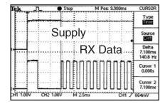
Figure 3: Turn-On Time from  $V_{CC}$
