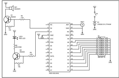
Figure 12: Basic Remote Control Receiver
