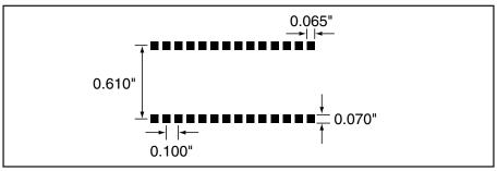
Figure 17: Recommended PCB Layout
