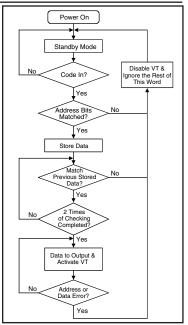
Figure 9: Decoder Flowchart
