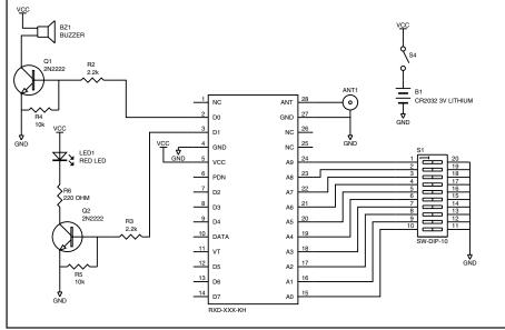
Figure 12: Basic Remote Control Receiver
