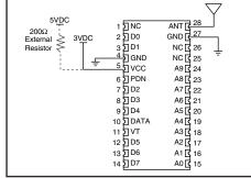
Figure 2: Test / Basic Application Circuit
