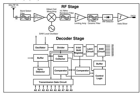
Figure 8: KH Series Receiver Block Diagram
