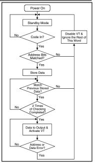
Figure 9: Decoder Flowchart
