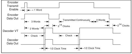
Figure 10: Encoder / Decoder Timing Diagram
