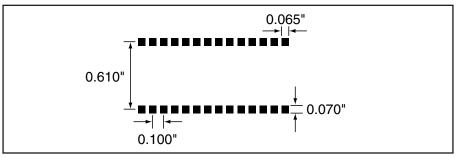
Figure 17: Recommended PCB Layout
