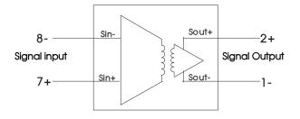
2.Schematic diagram of signal input and signal output(Ideal state)
