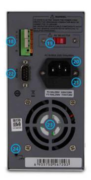
① LCD display ② Store shortcuts ③ Voltage setting key ④ Current setting key ⑤ Menu key ⑥ Keyboard lock ⑦ Output key ⑧ Rotary encoder ⑨ Shift right key ① Shift left key ① Return key ② Confirm key ③ Power switch ② Positive output terminal ⑤ Negative output terminal ⑥ GND terminal ① Output status indicator ⑧ Remote compensation terminal ② Input source selection terminal ② AC socket ② Fuse slot ② RS232 ② Fan ② Protected GND
