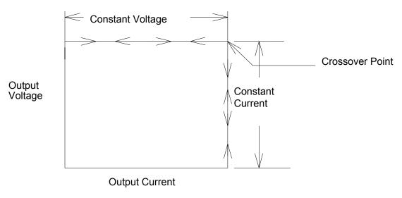
Figure 3 Constant Voltage vs. Constant Current Relation Diagram
