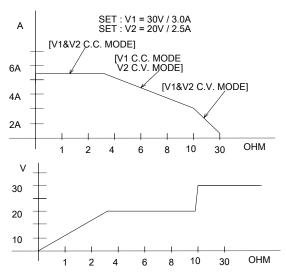
Figure 7 Parallel Voltage/Current Output vs. Load Change
