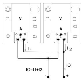
Figure 6 Parallel Connection Diagram
