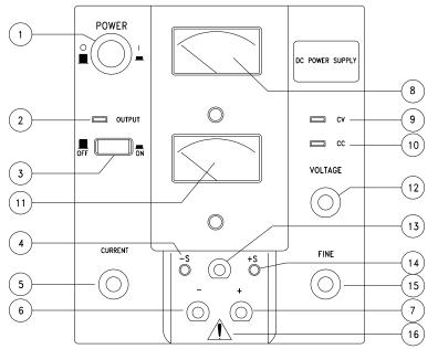
Front panel with analog meter for models 3203AR, 3302AR, 3303AR and 3601AR
