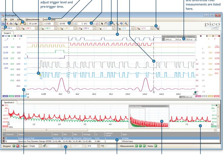
Movable axes: The vertical axes can be dragged up and down. This feature is particularly useful when one waveform is obscuring another. There's also an Auto Arrange Axes command.
