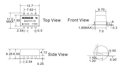
Note: All Pins on a 2.54mm pitch: all pin diameters are 0.50mm; all dimensions in mm.
