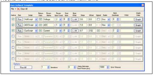
Create the Parameter Template by filling in each line. Each line is a single parameter, a value read converted to value displayed. The *inputs* below define how a particular parameter is interpreted.
