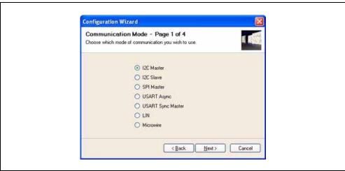
In this example, I<sup>2</sup>C Master Communication mode is selected. The Configuration Wizard Page 2 of 4, as shown in Figure 3-4, allows you to select the bus speed. A more comprehensive list of bus speeds can be chosen from the Configuration window by selecting <u>PICkit Serial Analyzer > Configure Communications Mode</u> from the menu bar.
