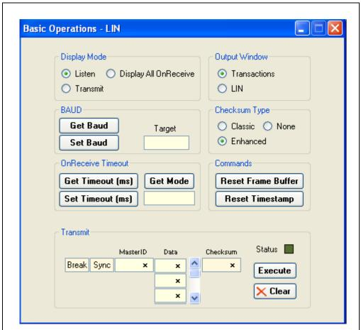
**Display Mode:** Determines when OnReceive data is displayed. Listen will display when the completed frame is different than the last frame, Transmit will not display data, and Display All will display all OnReceive data.
