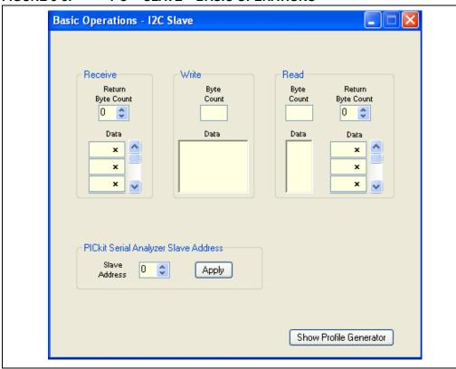
**Receive** responds to a basic Receive request from the master. In Return Byte Count, enter the number of bytes a Receive request will respond with, then enter the data to be returned in the data array. The Basic page limits you to eight bytes of returned data.
