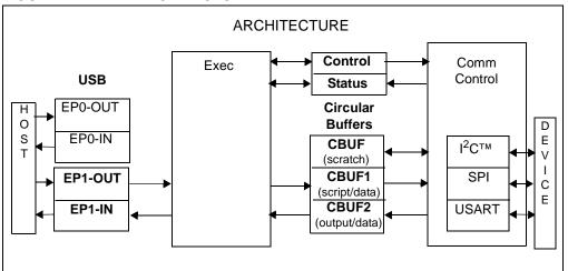
Data streams associated with PICkit™ Serial Analyzer are formatted with markers called "Tag" bytes. A Tag may be stand-alone or accompanied by data. As seen in Table 11-1, the data stream for each state controller has a set of associated Tag bytes defined in detail later in the document.
