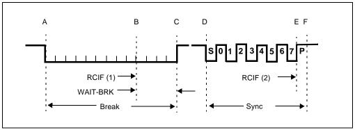
LIN specifications limit the baud rate to 20k (Reference the following table for examples).
