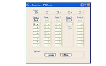
Once the WREN latch has been enabled, data can be written to the 25LC020A. Figure 7-6 shows that Group 0 has been disabled, and Group 1 enabled. Clicking on the **Execute** button will send the Write command (0x02), the memory address (0x00), followed by three bytes of data: 0xAA, 0xBB and 0xCC. The command will be logged in the Transactions window.
