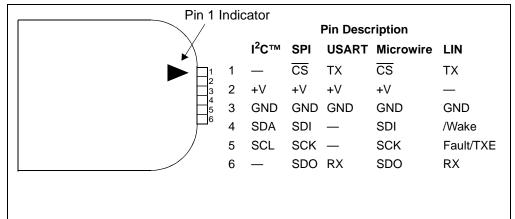
**Note:** The 6-pin header (0.100" spacing) accepts 0.025" square pins.
