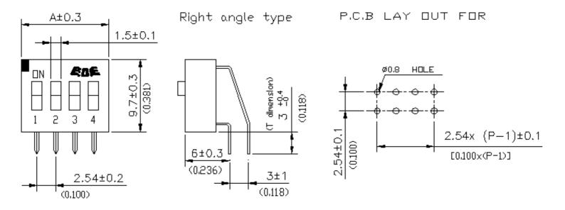
\*\* The 'T' dimension of the 1 position switch is 3.0±0.2
