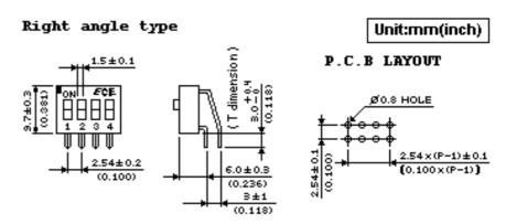
\*\* The "T" dimension of the 1 position switch is 3.0 ± 0.2
