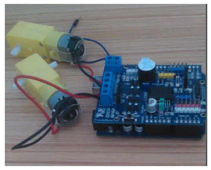
With wiring as the image shows, we can control forward rotation, reverse rotation, stop and the PWM speed of the two DC motors.
