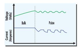
**Bulk:** This is the first charging stage where the battery at low charge stage, typically 10%, receives the majority of its charge. During this stage the battery brought to about 95% of its charger getting 100% of the available solar power.
