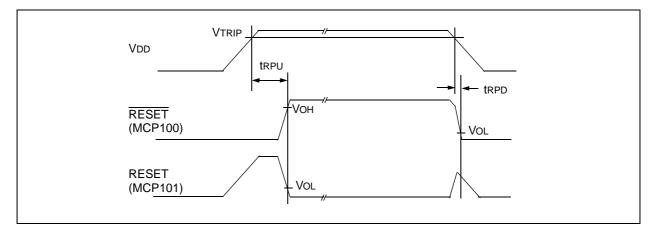
Figure 1-1: MCP100/101 Timing Diagram
