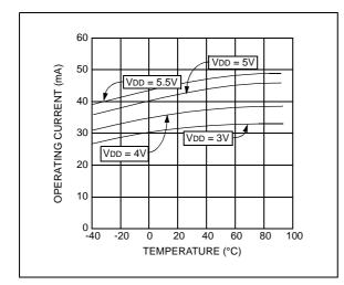
Figure 2-4: IDD vs. Temperature
