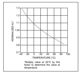
Figure 2-7: Normalized IOL vs. Temperature
