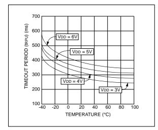
Figure 2-3: Typical tRPU vs. Temperature
