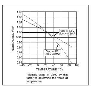
Figure 2-9: Normalized VOH vs. Temperature
