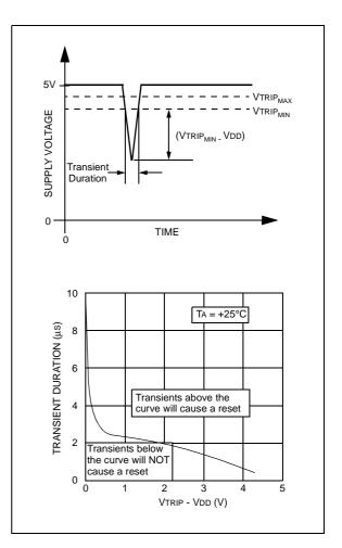
Figure 2-2: Typical Transient Response
