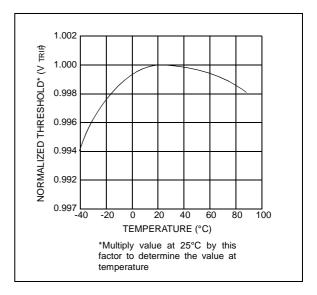
Figure 2-5: Normalized VTRIP vs. Temperature
