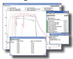
In addition to the monitor view, PicoLog can also display a graph, a spreadsheet and user notes. It can display them all at once, as shown here, or individually in any combination.
