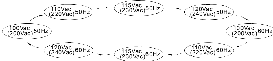
Figure 5.2: State Circulation Diagram of Output Voltage and Frequency
