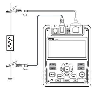
Figure 6. Low Resistance Measurement
