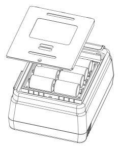
Figure 8. Battery Replacement
