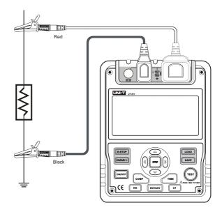
Figure 5. Insulation Resistance Measurement
