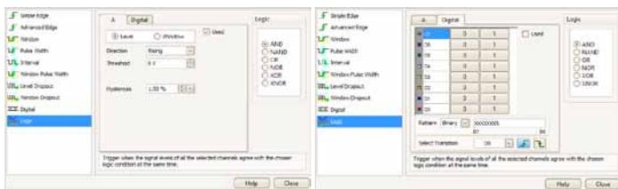
Digital triggering reduces re-arm delay and combined with the segmented memory allows the triggering and capture of events that happen in rapid sequence. Our Mask limit testing function can then scan through these waveforms to highlight failed waveforms for viewing in the waveform buffer.
