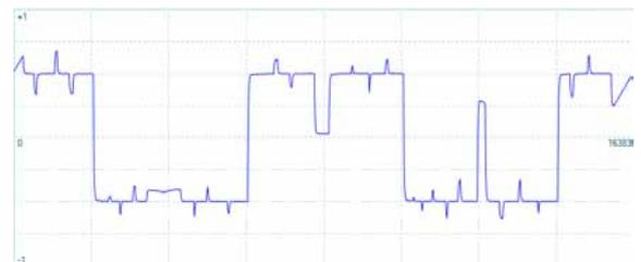
Also included is a fully programmable arbitrary waveform generator with a 8 k-sample buffer.
