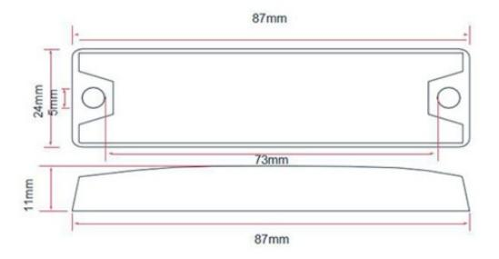
Size: 87×24mm, thickness 11mm, hole (diameter 5mm)
