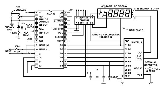
FIGURE 10. DRIVING LCD DISPLAYS
