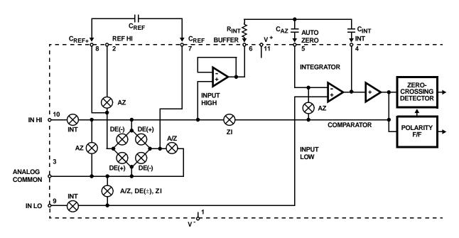
FIGURE 3. ANALOG SECTION OF ICL7135
