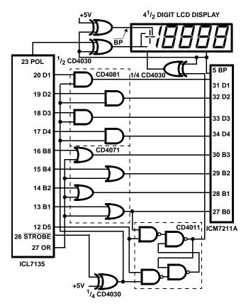
FIGURE 9. LCD DISPLAY WITH DIGIT BLANKING ON OVERRANGE
