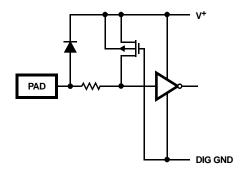
FIGURE 1. ICL7135 TEST CIRCUIT
