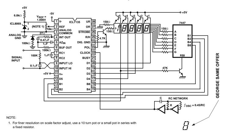
FIGURE 7. 41/2 DIGIT A/D CONVERTER WITH A MULTIPLEXED COMMON ANODE LED DISPLAY
