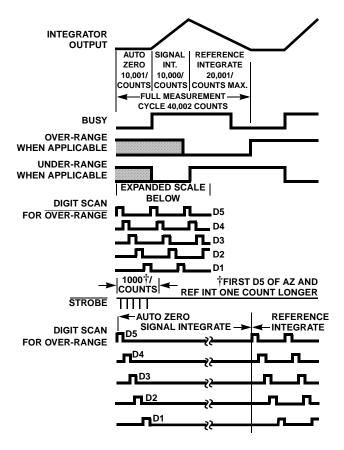
FIGURE 6. TIMING DIAGRAM FOR OUTPUTS
