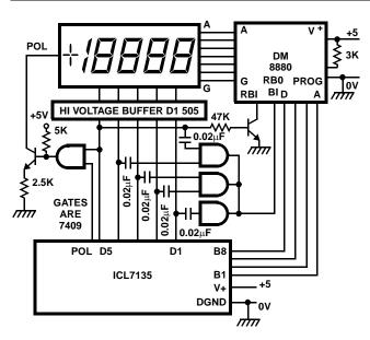
FIGURE 8. ICL7135 PLASMA DISPLAY CIRCUIT
