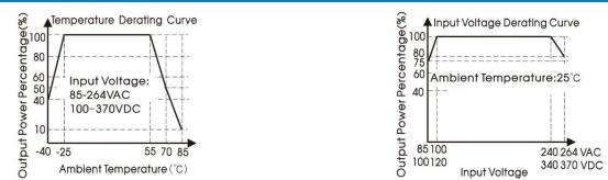
Note: ① With an AC input between 85-100V/240-264VAC and a DC input between 100-120V/340-370VDC, the output power must be derated as per temperature derating curves;
