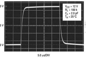
Figure 7. Error Amp Transient Response
