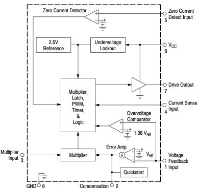
Figure 1. Simplified Block Diagram
