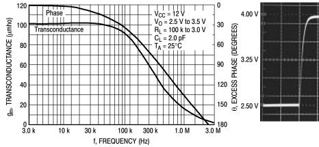
Figure 6. Error Amp Transconductance and Phase versus Frequency
