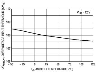
Figure 5. Overvoltage Comparator Input
