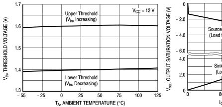
Figure 10. Zero Current Detector Input Threshold Voltage versus Temperature
