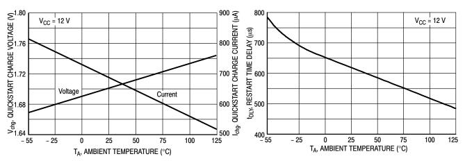
Figure 8. Quickstart Charge Current versus Temperature
