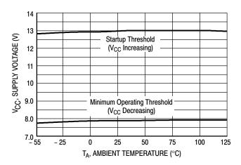
Figure 15. Undervoltage Lockout Thresholds versus Temperature
