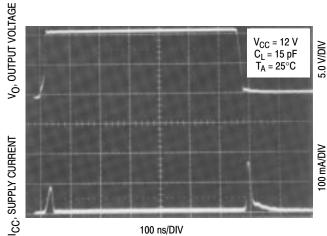
**Figure 13. Drive Output Cross Conduction**
