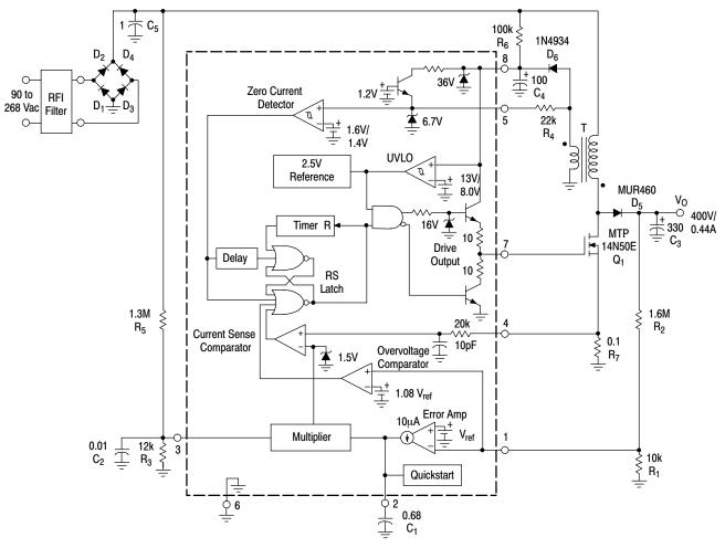
Figure 21. 175 W Universal Input Power Factor Controller
