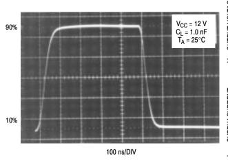
Figure 12. Drive Output Waveform
