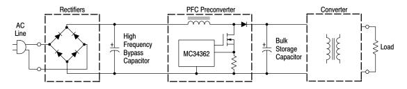
Figure 18. Active Power Factor Correction Preconverter
