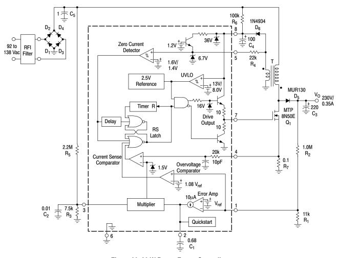
Figure 20. 80 W Power Factor Controller
