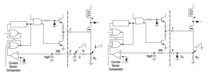
Figure 27. Current Waveform Spike Suppression
