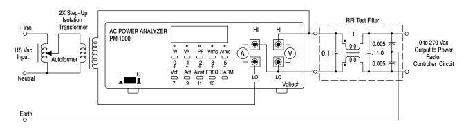
Figure 25. Power Factor Test Set-Up
