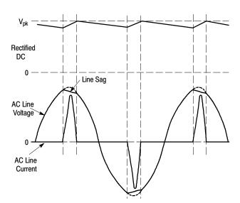
Figure 17. Uncorrected Power Factor Input Waveforms
