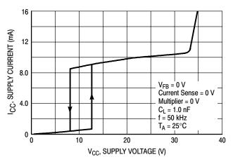
Figure 14. Supply Current versus Supply Voltage
