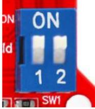
**Control Switch:** to control the serial connection between ESP8266 and arduino control board
