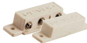
B182P (B1956) REED-ALARM SWITCH NC TYPE OPERATING GAP 3.5cm MAX
