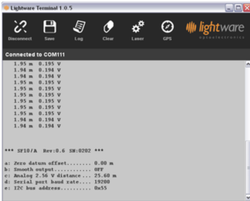
Figure 9 :: LightWare Terminal showing menu options
