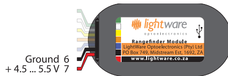
Figure 4 :: Regulated +5 V DC power supply connections
