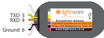
Figure 7 :: Serial interface connections
