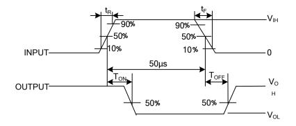
Note 1: Pulse width 50 $\mu$ s ,duty cycle 10% Output impedance 50 $\Omega$  t<sub>R</sub> 5ns, t<sub>F</sub> 10ns Note 2: See below
