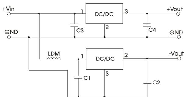
Fig. 3 Positive and Negative output parallelling application circuit
