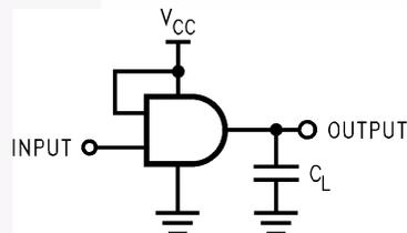
C<sub>L</sub> includes load and stray capacitance
