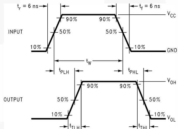
**Figure 3. AC Waveforms**
