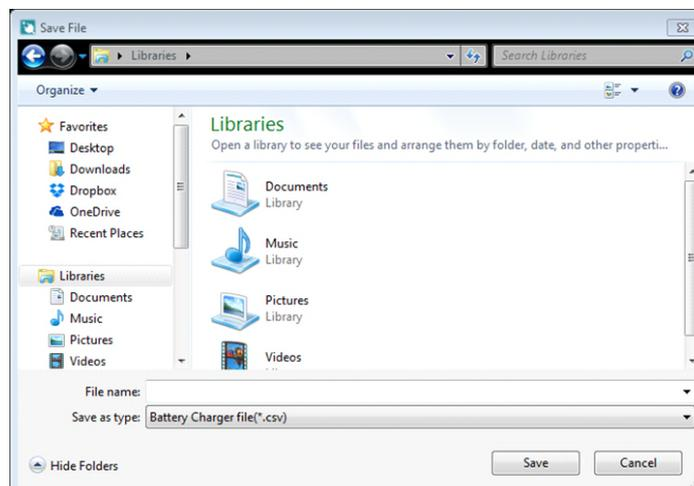
Type a file name (This SBPSetting.csv is an example of explanation, shown as A marked in red in the picture below) and then click “Save” (as B) to save the current settings.
