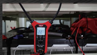
DC current test of Battery modules
