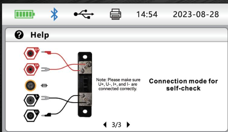
The instrument can perform self-tests using an accessory standard resistor to verify measurement accuracy and ensure data reliability.
