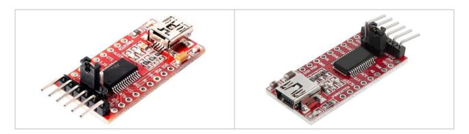
The product in this image is a **USB to TTL Serial Adapter Board**.
