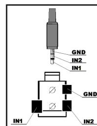
The connector can interface standard 3.5 mm phone connector (also known stereo plug or audio plug).
