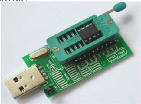
2: Insert the programmer into the USB port of the computer and open "CH341A programmer 1.17" Programming software in. Select the chip, you can program and erase the chip.25 series chip programming (P/S end jumper closed, programming method is the same as 24 series) Place the chip as shown below:
