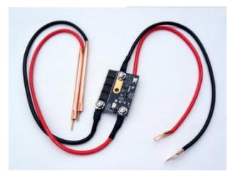
Spot welding through a principle that large current local heating or cooling need enough current to supply. The welding current approx 90-130A, which is more than enough to welding common 0.1mm-0.12mm Input wire Circuit board Output wire and welding pen Jal or greater than 150A.
