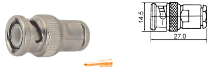
M5541T BNC male clamp type gold-pin (RG58U/59U/6AU/8AU) teflon insulation
