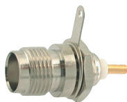
M5755 TNC female bulkhead crimp type gold-pin (RG58U/59U)
