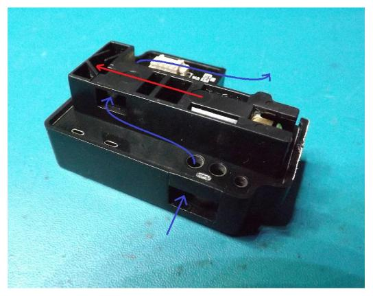
Fig. 4: Air flow (blue) and laser beam (red)
