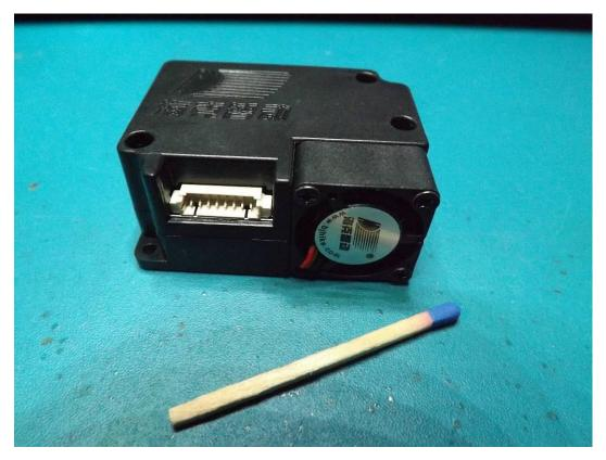
Fig. 2: Fan (air outlet) and connector
