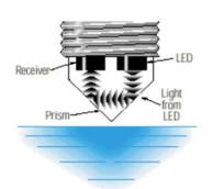
Liquid below the sensing prism.
