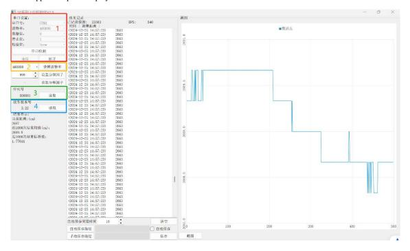
Area 1: Set the corresponding serial port parameters and click Connect
