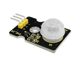
The Pyroelectric infrared motion sensor can detect infrared signals from a moving person or moving animal, and output a switching signal.
