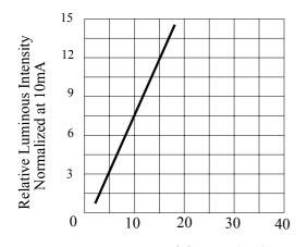
Forward Current (mA) Fig.5 RELATIVE LUMINOUS INTENSITY VS. FORWARD CURRENT
